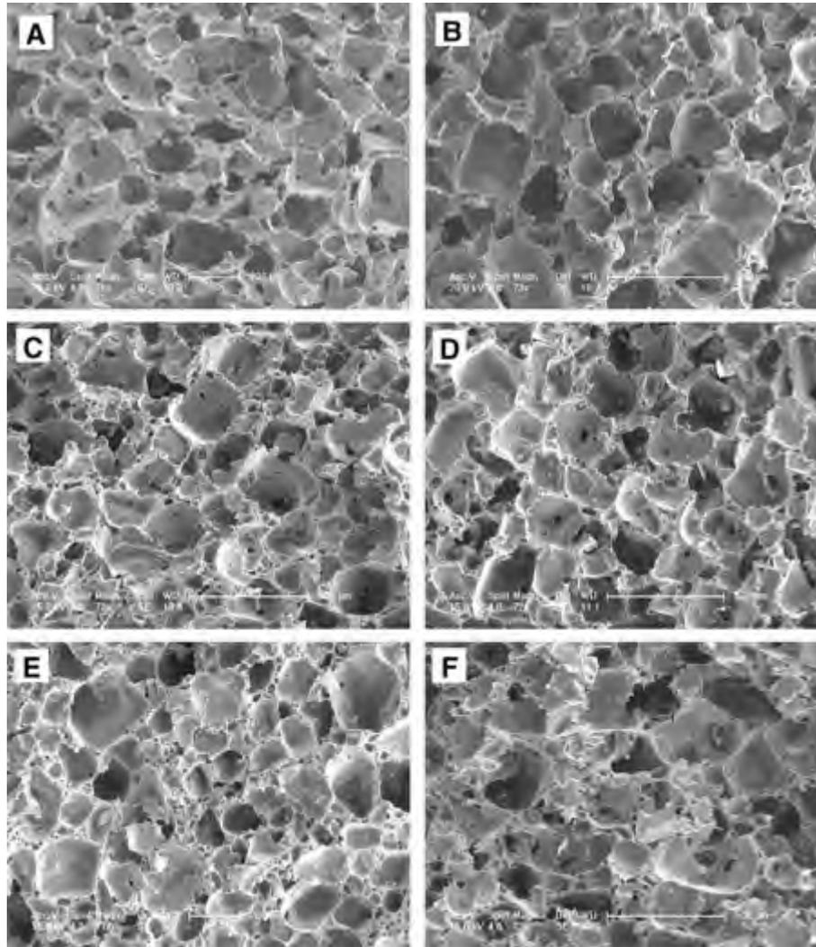
Fig. 1. SEM micro-photographs of porous scaffolds of: PLGA (A), 5 wt.% op-HA/PLGA (B), 10 wt.% op-HA/PLGA (C), 20 wt.% op-HA/PLGA (D), 40 wt.% op-HA/PLGA (E) and HA/PLGA (F) fabricated with the melt-molding particulate leaching method. Scale bar lengths are 200  $\mu\text{m}$  (A and E), 500  $\mu\text{m}$  (B, C, D and F).
