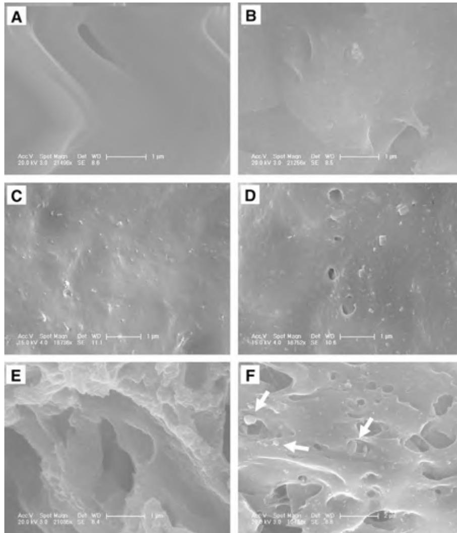
Fig. 3. The surface topography of the pore walls of the porous scaffolds of: PLGA (A), 5 wt.% op-HA/PLGA (B), 10 wt.% op-HA/PLGA (C), 20 wt.% op-HA/PLGA (D), 40 wt.% op-HA/PLGA (E) and 10 wt.% HA/PLGA (F). Scale bar lengths are 1 µm (A–E) and 2 µm (F).
