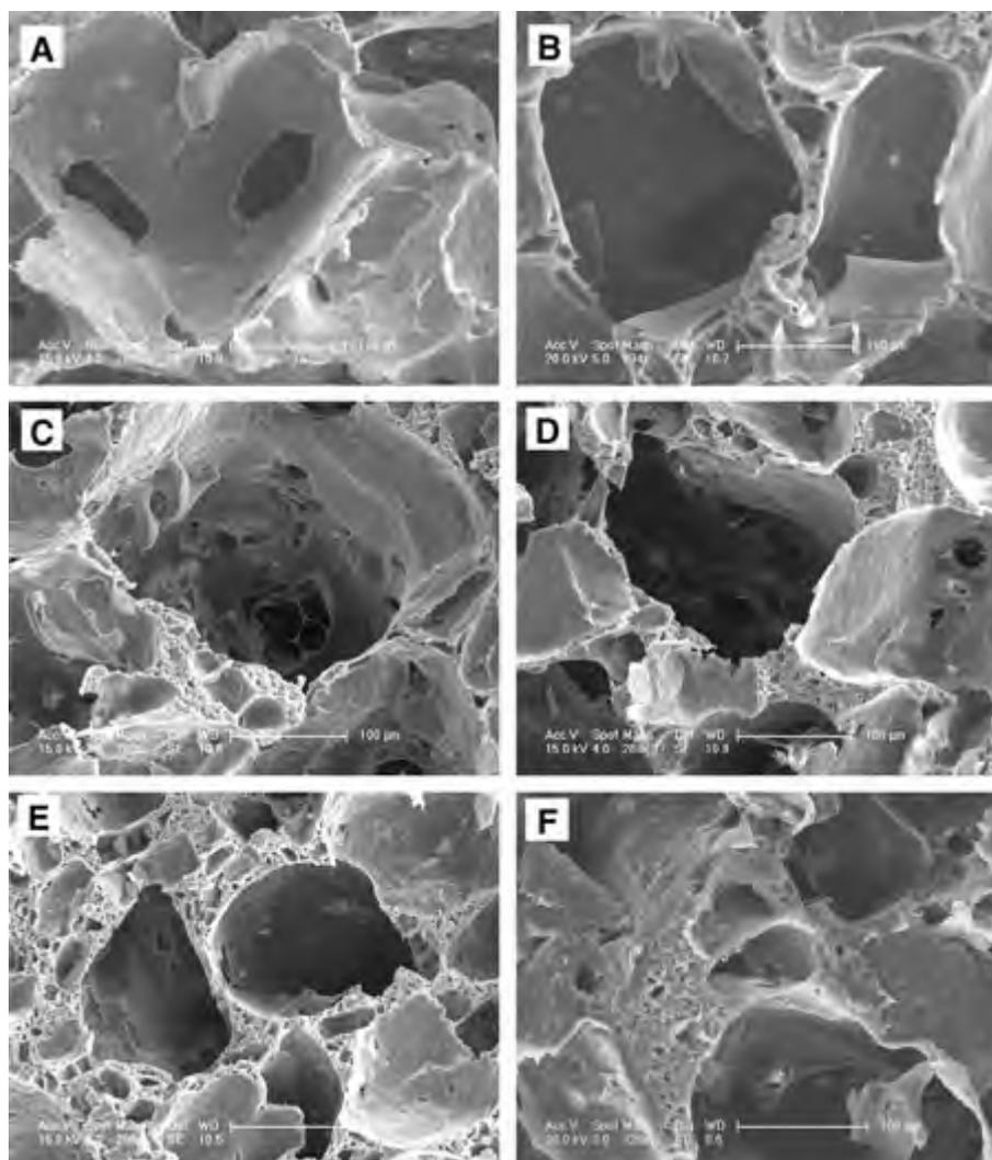
Fig. 2. SEM micro-photographs of porous scaffolds of: PLGA (A), 5 wt.% op-HA/PLGA (B), 10 wt.% op-HA/PLGA (C), 20 wt.% op-HA/PLGA (D), 40 wt.% op-HA/PLGA (E) and HA/PLGA (F) fabricated with the melt-molding particulate leaching method. Scale bar lengths are 100 µm.
