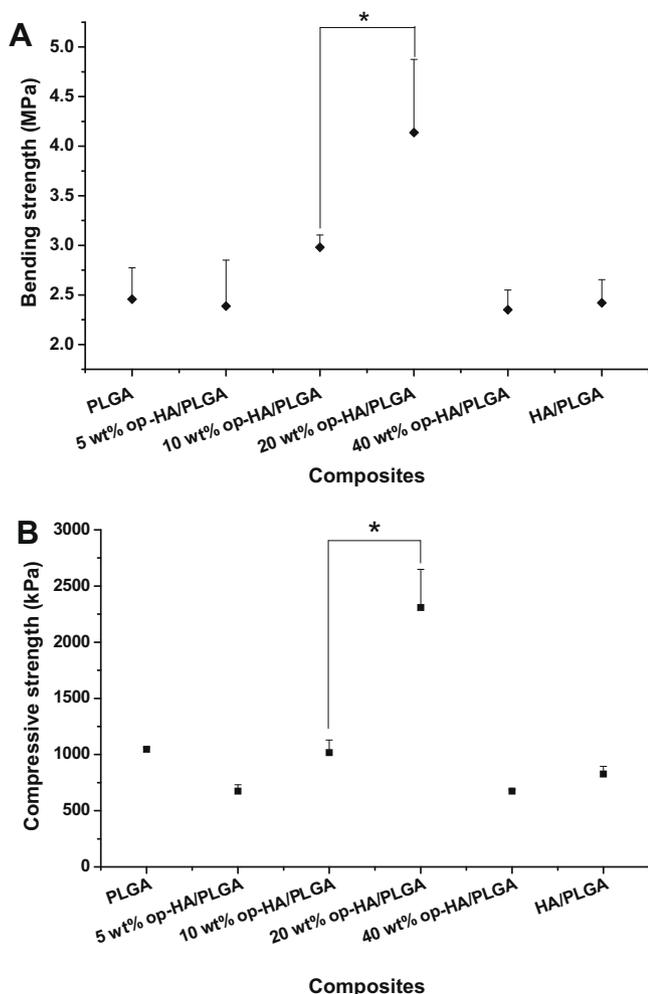
Fig. 4. Dependence of bending strength (A) and compressive strength (B) on the filler of op-HA or HA content in the composite scaffolds.
