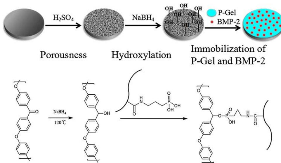
Scheme 1. Schematic diagram illustrating the processes of modification on PEEK films.
