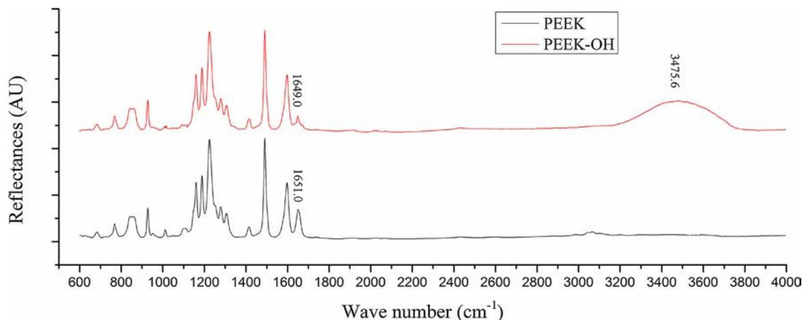
**Fig. 2.** FT-IR spectra of PEEK (black) and PEEK-OH films (red). (For interpretation of the references to colour in this figure legend, the reader is referred to the web version of this article.)
