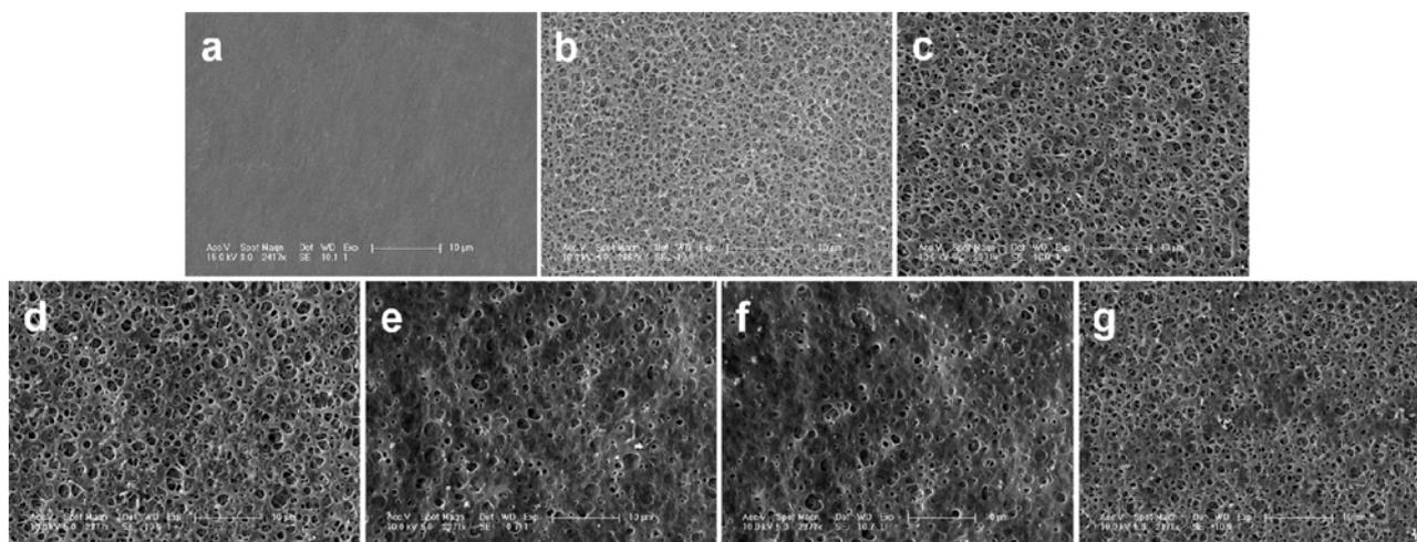
**Fig. 1.** ESEM images of un-PEEK (a), PEEK (b), PEEK-OH with 0.1% P-Gel (c), PEEK-OH with 1% P-Gel (d), PEEK-OH with 2% P-Gel (e), PEEK-OH with 4% P-Gel (f), and PEEK with 2% P-Gel (g). All scale bar length are 10  $\mu\text{m}$ .
