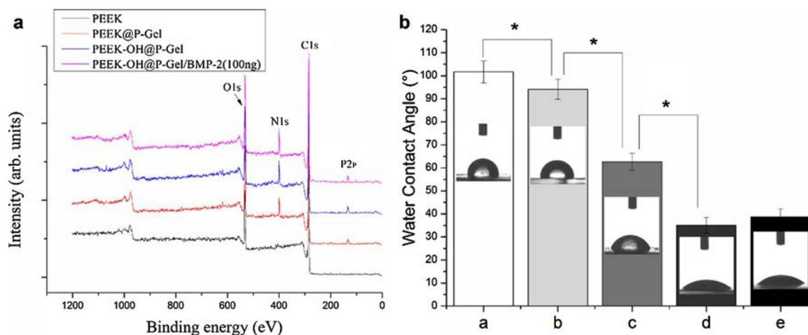
**Fig. 3.** (a) XPS spectra of PEEK (black), PEEK@P-Gel (red), PEEK-OH@P-Gel (blue), PEEK-OH@P-Gel/BMP-2 (100 ng) (purple). (b) Water contact angle of un-PEEK (a), PEEK (b), PEEK-OH (c), PEEK-OH@P-Gel (d), PEEK-OH@P-Gel/BMP-2 (100 ng) (e). \* indicates significant differences ( $P < 0.05$ ). (For interpretation of the references to colour in this figure legend, the reader is referred to the web version of this article.)
