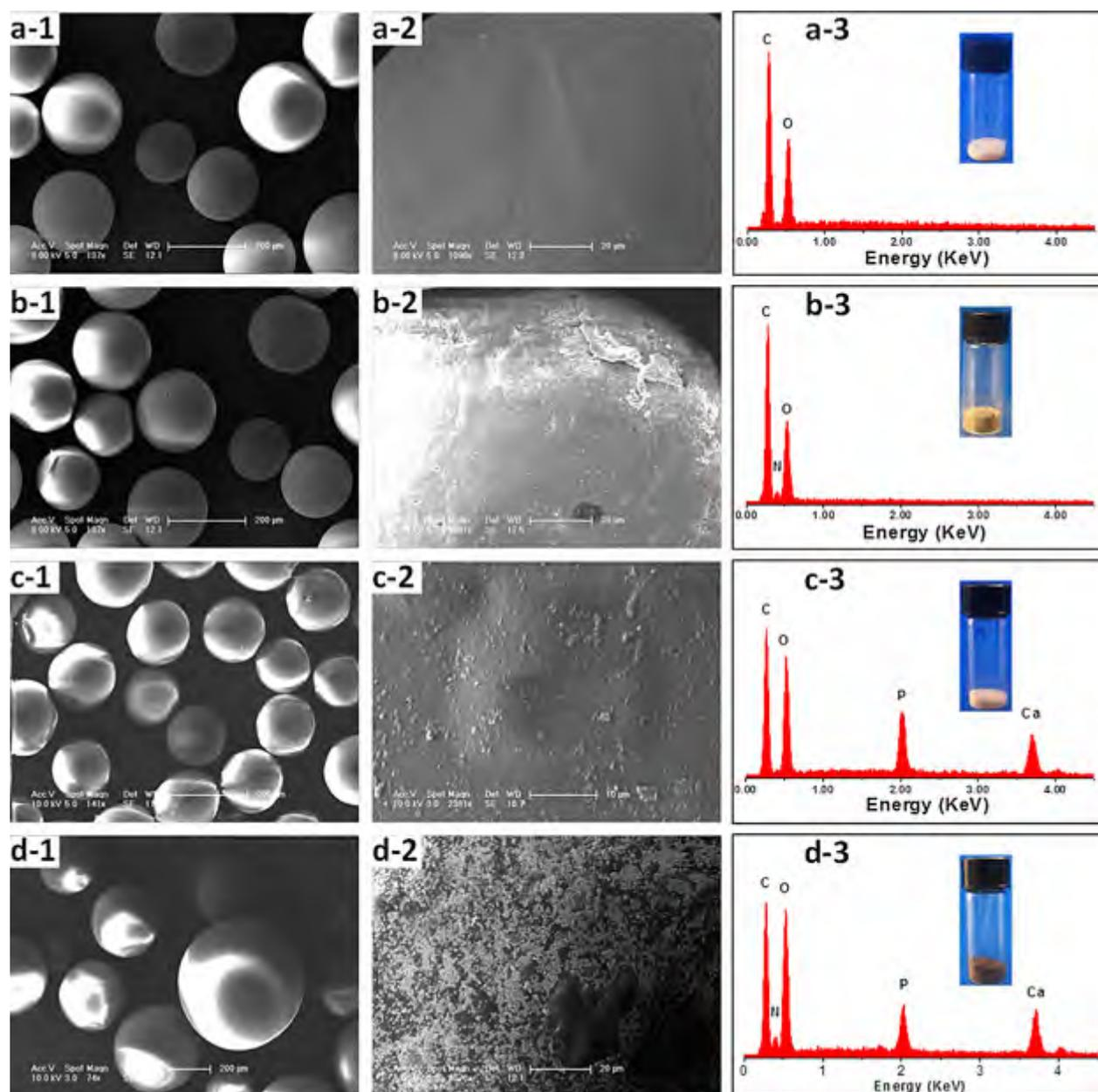
**Figure 1.** SEM images (1–2) and EDX (3) of PLGA (a), pDA @ PLGA (b), PLGA/HA (c), and pDA @ PLGA/HA (d) microcarriers. Bar lengths are 200 μm (a-1, b-1, c-1, and d-1), 20 μm (a-2, b-2, and d-2) and 10 μm (c-2).
