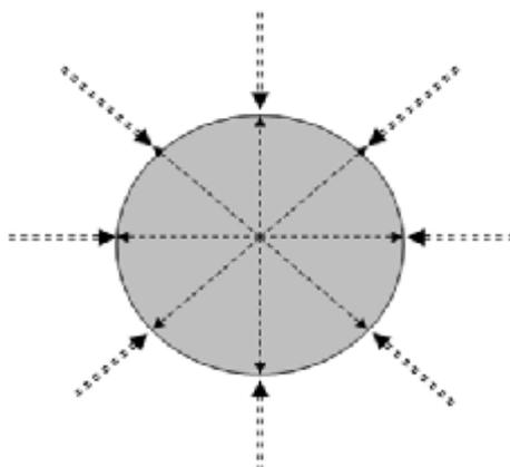
**Scheme 1** Relationship between porous structures and pore growing directions in the one phase solution freeze-drying method
