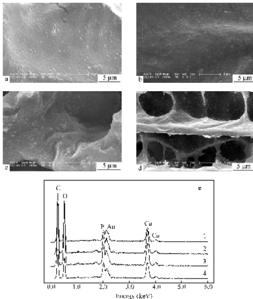
**Fig. 3** Pore wall surface topography (a–d) and EDX curves (e) of the porous scaffolds fabricated with the freeze-dry method by different freezing temperatures: 4°C (a and e-1), –20°C (b and e-2), –80°C (c and e-3) and –196°C (d and e-4)
