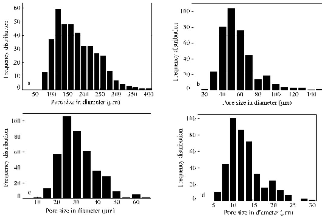
**Fig. 2** Frequency distribution of pore diameters of op-HA/PLGA scaffolds based on different freezing temperatures: 4°C (a), -20°C (b), -80°C (c) and -196°C (d)
