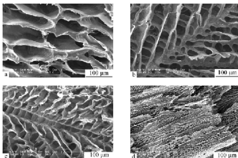
**Fig. 1** SEM micrographs of transverse sections of the nanocomposite scaffolds of op-HA/PLGA with a honeycomb monolith structure fabricated with freezing temperatures of 4°C (a), -20°C (b), -80°C (c) and -196°C (d)
