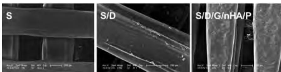
**Figure 2.** Scanning electron micrographs (SEM) of PLA scaffold (S), dopamine-modified scaffold (S/D), and ponicin-immobilized scaffold (S/D/G/nHA/P).
