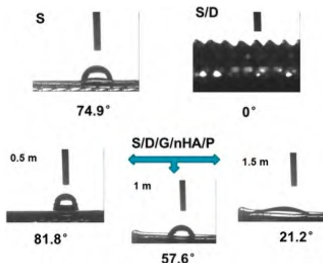
**Figure 3.** Wettability assessment of different scaffolds by water contact angle detection.
