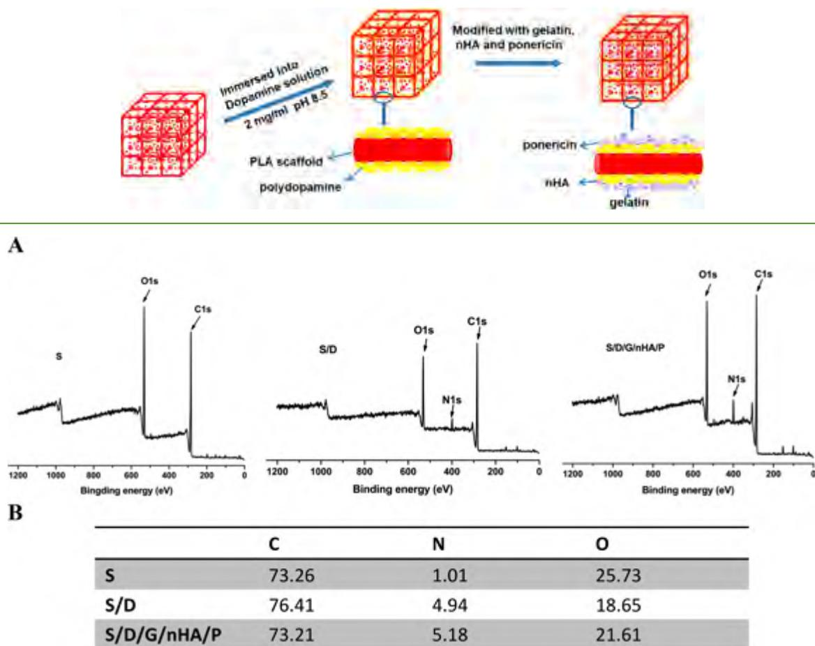
**Figure 1.** XPS spectra (A) and surface chemical composition (B) of untreated PLA scaffold (S), dopamine-modified scaffold (S/D), and ponicin-incorporating scaffold (S/D/G/nHA/P).
